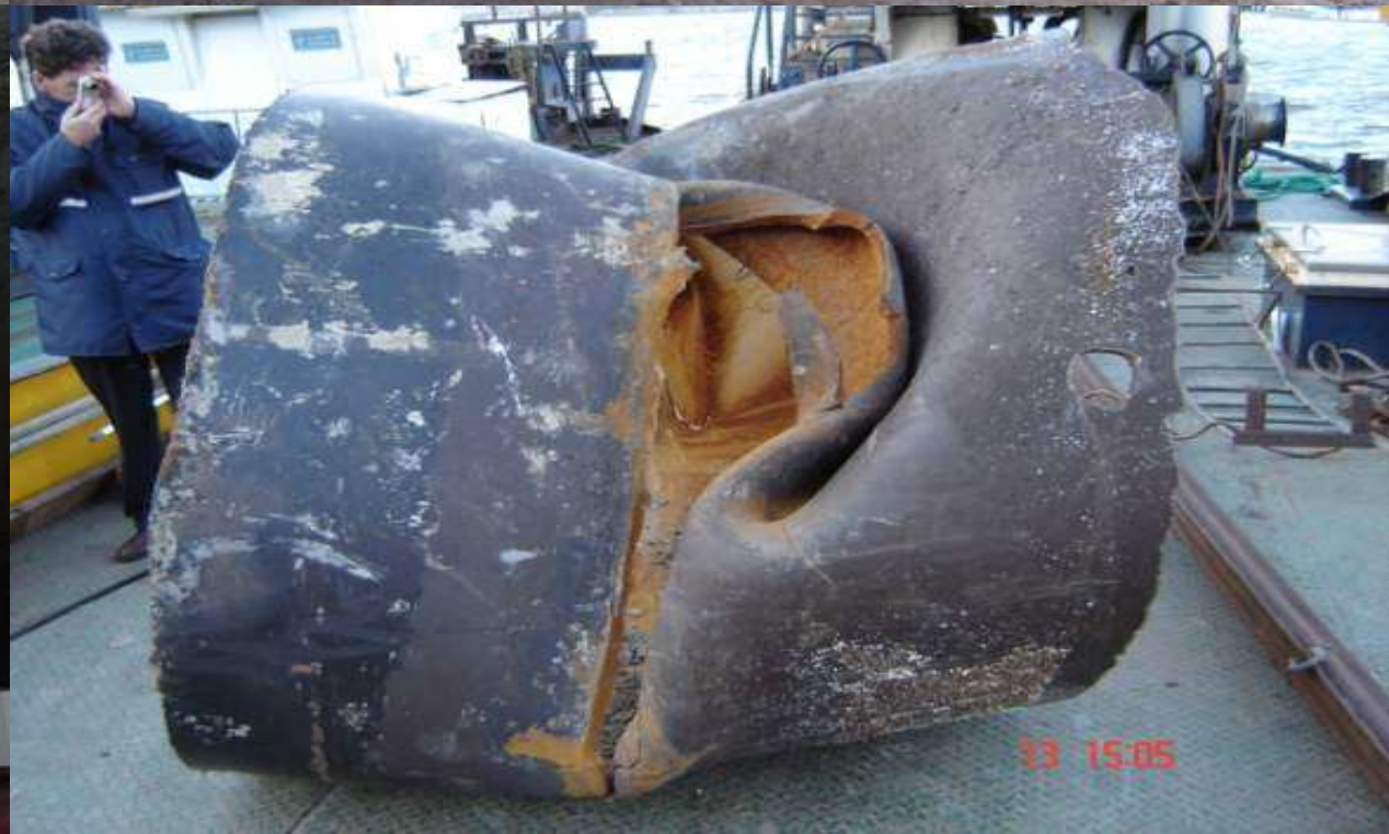
Local buckling empty tube (inwards)
